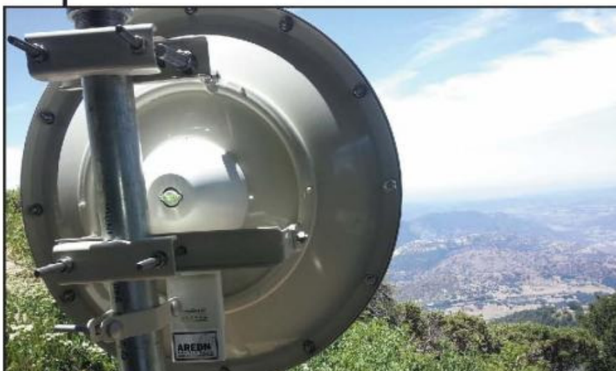
Figure 1. A Ubiquiti Rocket M3 AREDN™ node. On these frequencies, line of sight is important, so long-haul
