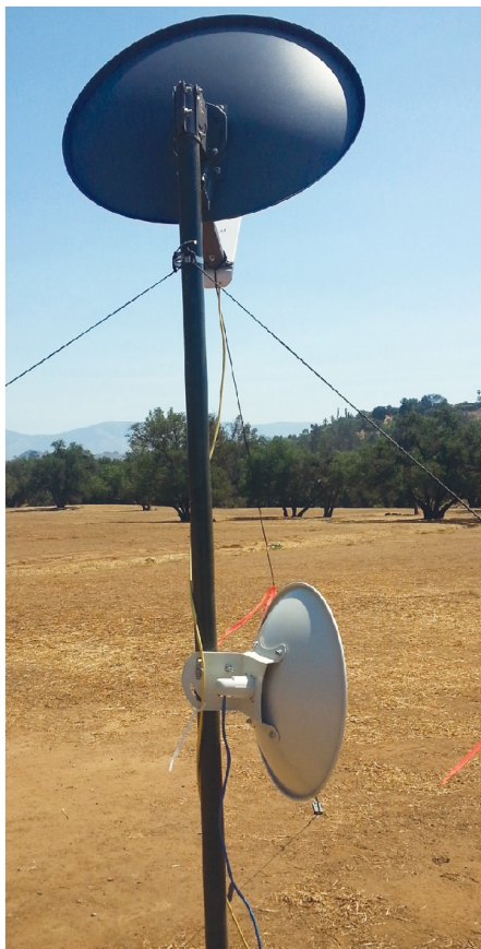
Figure 3 — This relay node shows a gain antenna pointed to a backbone node and another pointed to a deployed node at a shelter site. [Andre Hansen, K6AH, photo]
